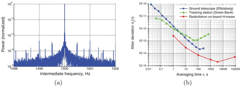
Fig. 2. Frequency stability of the 8.4 GHz RadioAstron downlink signal. (a) Phase-stopped signal spectrum (data recorded by the Effelsberg telescope, 2015/11/19). (b) Comparison of the frequency stability in terms of the Allan deviation of the signal recorded by a radio telescope (blue, circles) and a tracking station (green, diamonds). Allan deviation of the on-board H-maser obtained during laboratory tests (red, squares).
