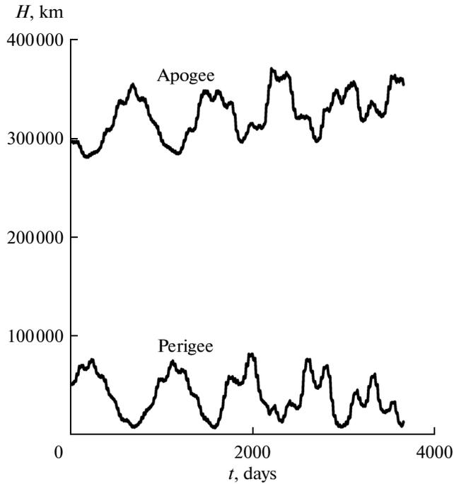
Fig. 2. Evolution of perigee height  $H_\pi$  and apogee height  $H_a$  of the orbit.
