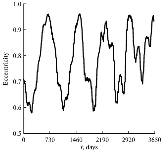
Fig. 3. Evolution of eccentricity of SRT orbit.
