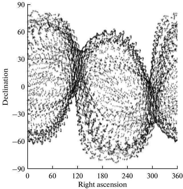
Fig. 1. Evolution of direction of the Earth–SRT vector onto the celestial sphere.
