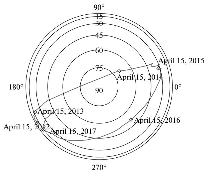
Fig. 5. Evolution of the projection of direction of a normal vector to the orbit plane onto the celestial sphere.
