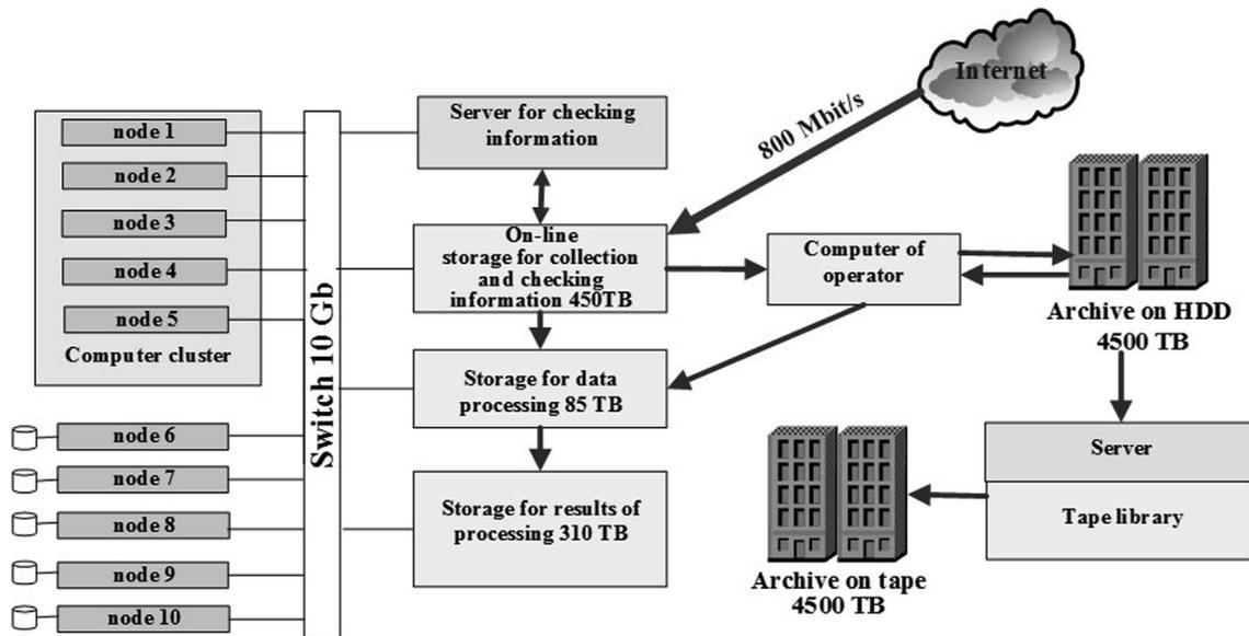
Fig. 5. Computer complex and data storage operation diagram.
