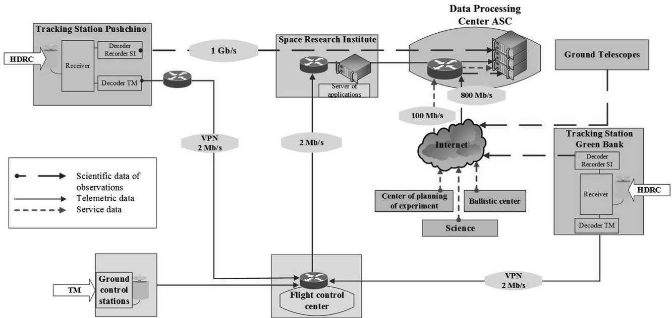
Fig. 6. Data Processing Center communication channels (SI – scientific information, TM – telemetry information, HDRC – High Data Rate Communication radio link).
