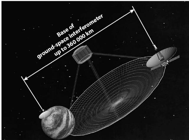
Fig. 1. Configuration of the RadioAstron space-ground interferometer.
