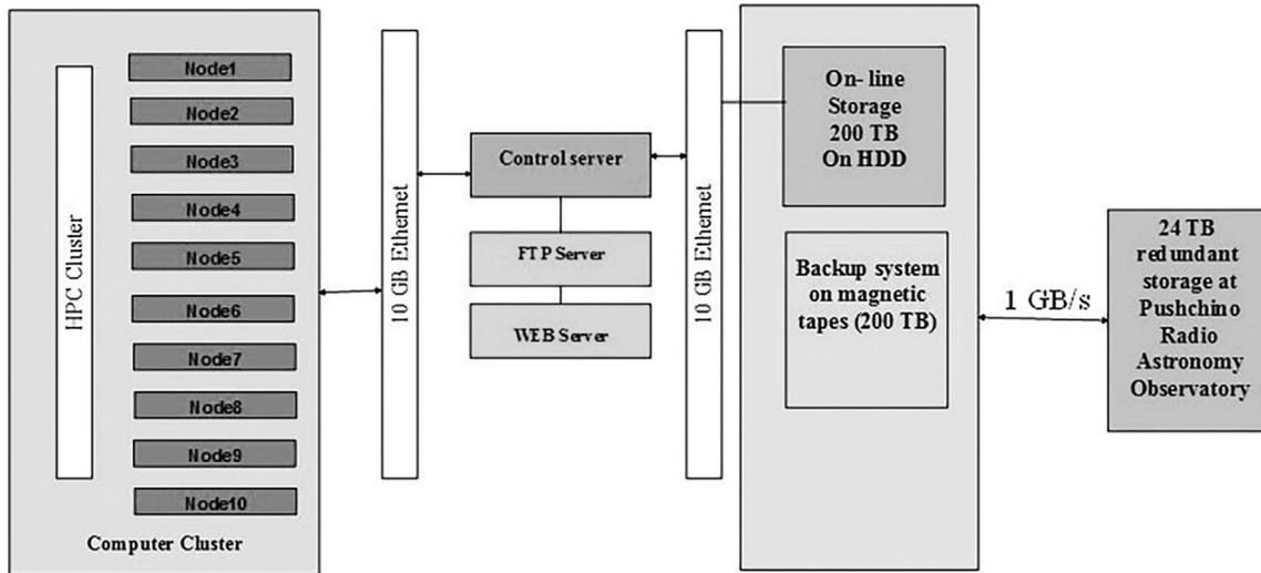
Fig. 4. Scheme of computer complex and storage operation.
