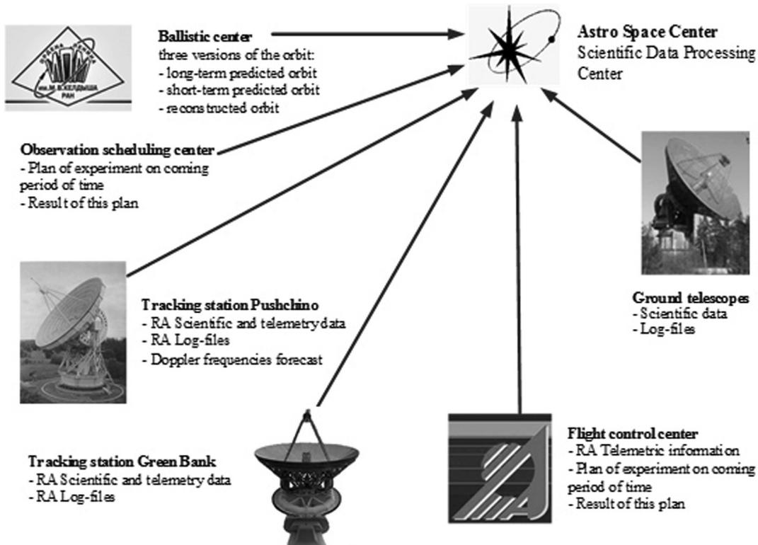
Fig. 2. Scheme of information exchange in the RadioAstron project.
