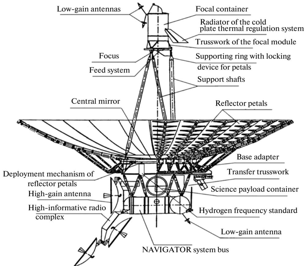
**Fig. 1.** Arrangement of the SRT and Navigator bus.
