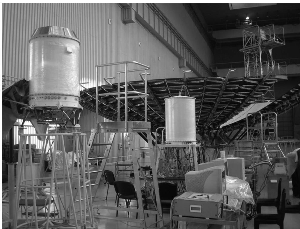
Fig. 4. The focal (left) and science payload (right) containers of the SRT.
