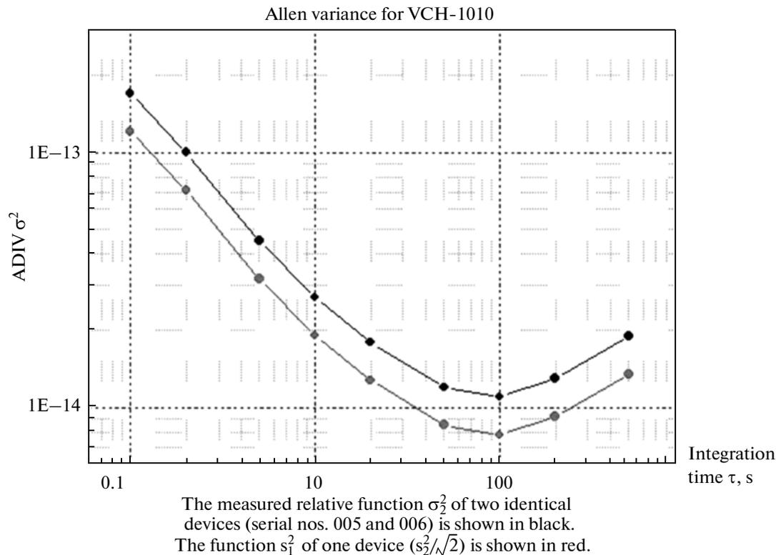
**Fig. 9.** Stability analysis of the frequency standard for the SRT.
