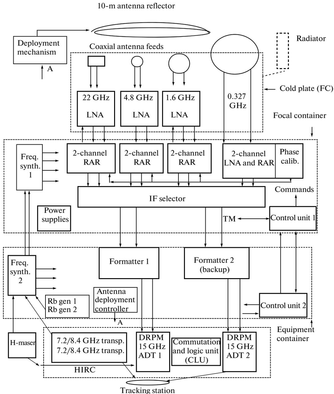
**Fig. 2.** The block-diagram of the SRT. LNA, low noise amplifier; FC, focal container with the feed system and LNA; RAR, radio astronomy receiver; IF, intermediate frequency; TM, telemetry information; Rb gen 1, 2; rubidium generators; H-maser, hydrogen generator (2 sets); HIRC, high-informative radio complex; 7.2/8.4 GHz transp., input-to-output (7.2 to 8.4 GHz) frequency transponder; DRPM, double phase manipulator; ADT 1, 2; Astronomical data transmitters with 15 GHz carrier frequency.
