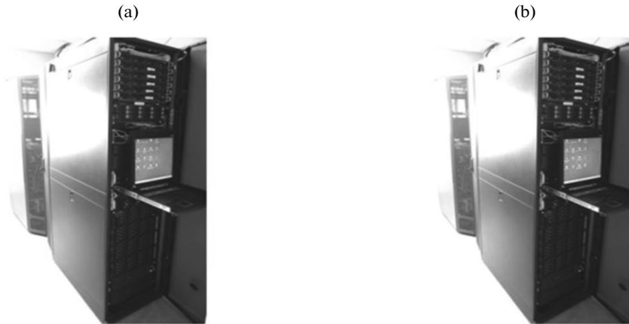
Fig. 3. Computing cluster with ten servers (performance of 1 TFLOP/s): (a) data storage with capacity of 220 TB; (b) backup device.
