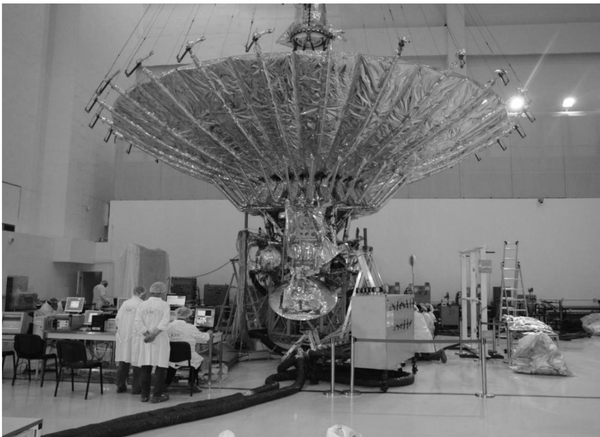
Fig. 3. Multitask tests of the SRT and the Navigator bus. The reflector is unfolded. (NPO Lavochkin, June 2011).
