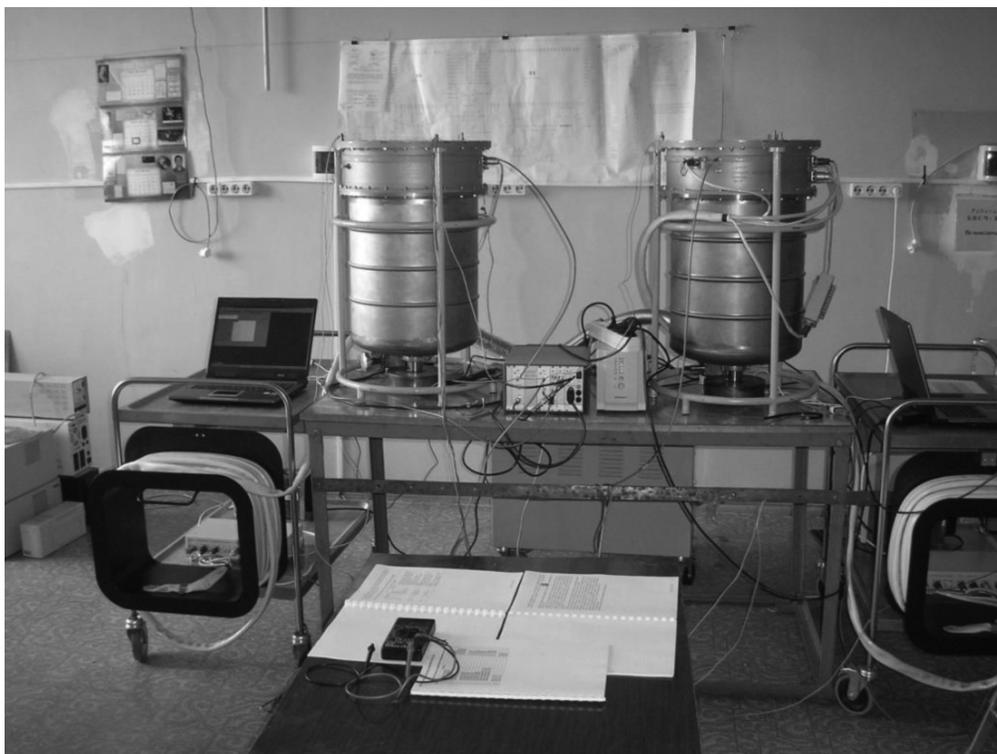
**Fig. 5.** Hydrogen frequency standards (masers) developed for the Radioastron project at the ZAO Vremya-Ch (Nizhni Novgorod).
