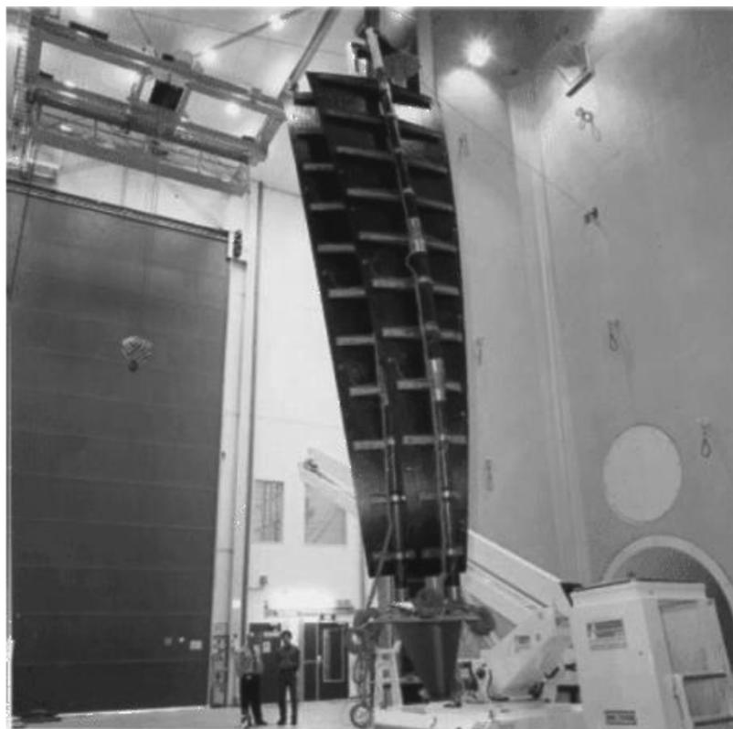
**Fig. 6.** Tests of individual carbon fiber petals of the SRT antenna (ESA, The Netherlands, Noordwijk, 1994).
