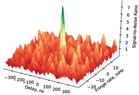
**Figure 3:** Interferometric signal from the quasar 0748+126 detected between RadioAstron and GBT (K-band) at the projected baseline of  $4.3 D_{\oplus}$ . The plot shows the signal to noise ratio as a function of residual delay and rate after delay-model subtraction and fringe fitting.
