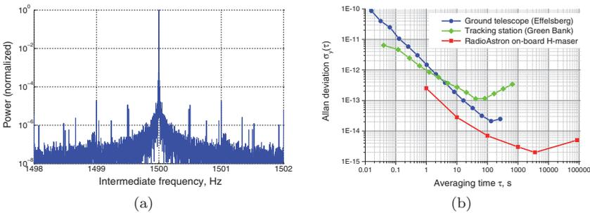
Fig. 2. Frequency stability of the 8.4 GHz RadioAstron downlink signal. (a) Phase-stopped signal spectrum (data recorded by the Effelsberg telescope, 2015/11/19). (b) Comparison of the frequency stability in terms of the Allan deviation of the signal recorded by a radio telescope (blue, circles) and a tracking station (green, diamonds). Allan deviation of the on-board H-maser obtained during laboratory tests (red, squares).
