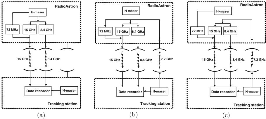
Fig. 1. On-board hardware synchronization modes. (a) “H-Maser”. (b) “Coherent”. (c) “Semi-Coherent”. Note that, due to a fixed architecture of the RadioAstron on-board radio system, the 8.4 GHz tone and the carrier of the 15 GHz data link must use one and the same reference signal at any given time: either from the on-board H-maser or from the tracking station uplink.
