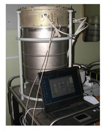
Fig. 3. One of the RadioAstron's on-board H-maser units undergoing laboratory tests, Moscow, Astro Space Center of P.N. Lebedev Physical Institute, July 2008.
