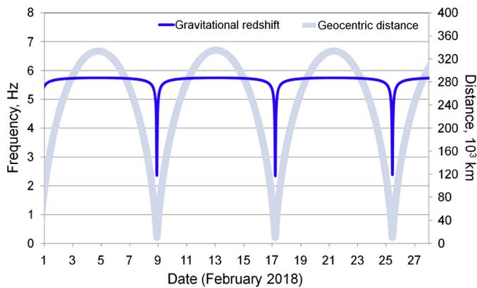
Fig. 2. Variation of the gravitational frequency shift of the 8.4 GHz downlink signal along the orbit during a low perigee epoch.
