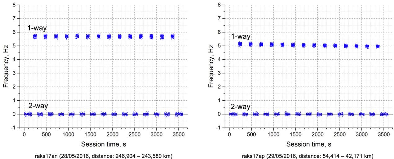
Fig. 6. Residual frequencies of the 1- and 2-way 8.4 GHz signals measured with the Onsala 20-m telescope. The 1-way frequency residuals are not corrected for the gravitational redshift. This makes the variation of the gravitational frequency shift between the two sessions clearly visible (varying from 5.69 Hz to 4.96 Hz).
