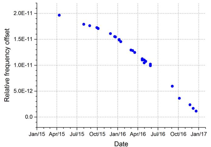
Fig. 3. Frequency drift of the RadioAstron on-board H-maser relative to the H-maser at the Green Bank TS.
