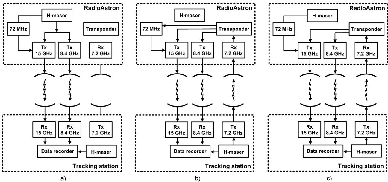
Fig. 4. Operation modes of the RadioAstron radio links: a) “H-Maser” (1-way); b) “Coherent” (2-way); c) “Semi-Coherent” (2-way).
