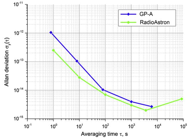
Fig. 1. Comparison of the frequency stability of the RadioAstron VCH-1010 [12] and GP-A VLG-10 [13] H-masers in terms of the Allan deviation.
