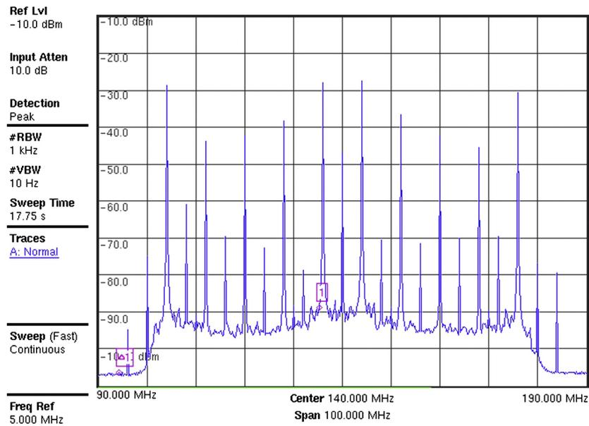
Fig. 5. Spectrum analyzer screenshot, showing the signal spectrum of the 15 GHz data downlink in the “Test-2” mode of the on-board formatter.
