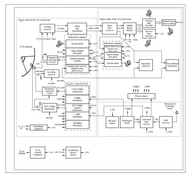
Fig. 3. Stuctural schematic of the ground tracking station in Pushchino.
